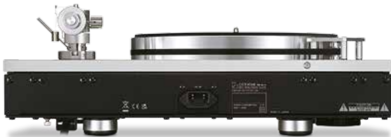
ABOVE: The four heavy-duty insulating feet are clearly visible here, each offering some 5mm of level adjustment. The tonearm lead connects via a DIN plug under the deck and is clamped in place for strain relief. The IEC mains inlet is gold-plated!
