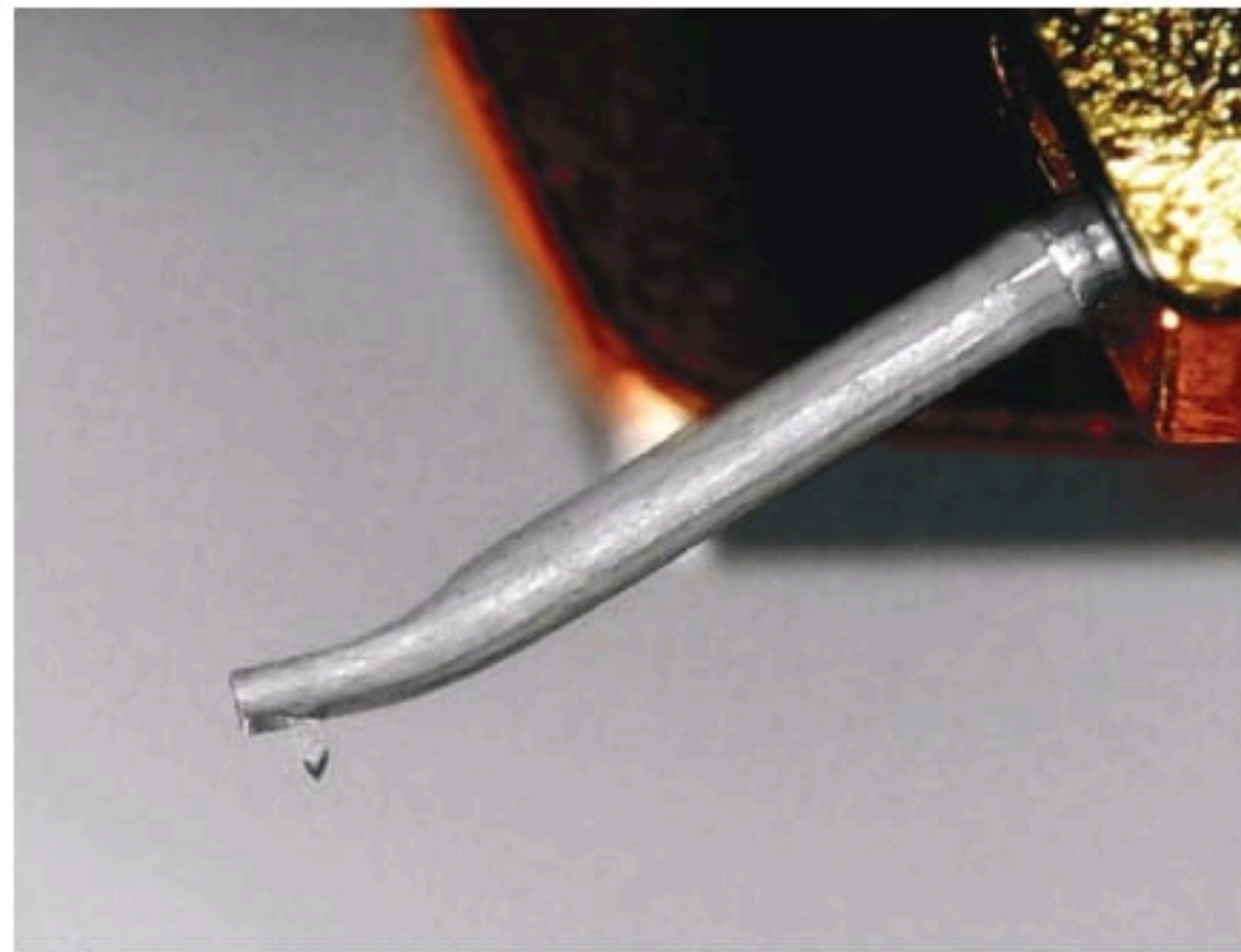
A conventional parallel sided aluminium alloy tube, crimped and bent at the end, a common manufacturing technique used on inexpensive cartridges.
