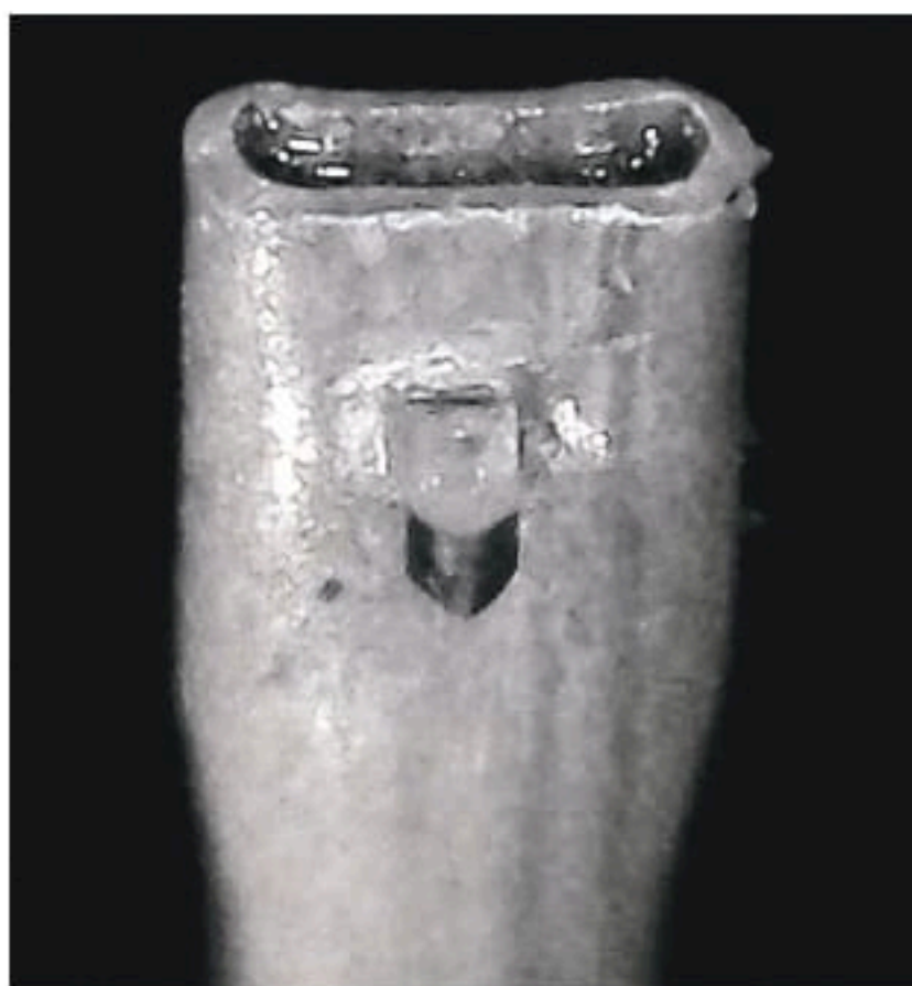
The stylus has a rectangular shank for accuracy of orientation on the cantilever. Note how the alloy tube has been crimped to provide a flat surface.
