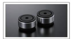
In order to maintain horizontal alignment, the PD-191A incorporates special damping rubber with excellent temperature characteristics and resistance to long-term deterioration into our originally designed, large-diameter insulator legs that can each be level adjusted up to 5mm in height to prevent the transmission of feedback and external vibrations.
