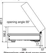
Dimensions with dust cover open [all dimensions are in millimeters]
