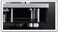
The underslung suspension structure, in which the main components are attached to a 15mm thick aluminum plate, has succeeded in achieving both high rigidity and damping performance. Also, by mounting the motor drive system and power transformer on an extra thick bottom plate, insulated with damping rubber, delicate signal pickup is protected from external vibrations, greatly improving the mechanical S/N ratio (rumble) and feedback resistance.
