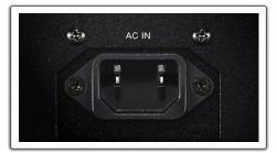
The AC inlet is gold-plated to reduce contact resistance and the entire terminal has been improved and reverse mounted in order to support a heavyweight AC cable.
