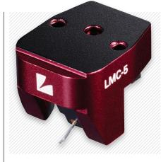
and an adhesive bond using epoxy resin. The cart's 4-nines, high-purity copper-coil windings consist of urethane-enameled piano wire 30µm thick.
