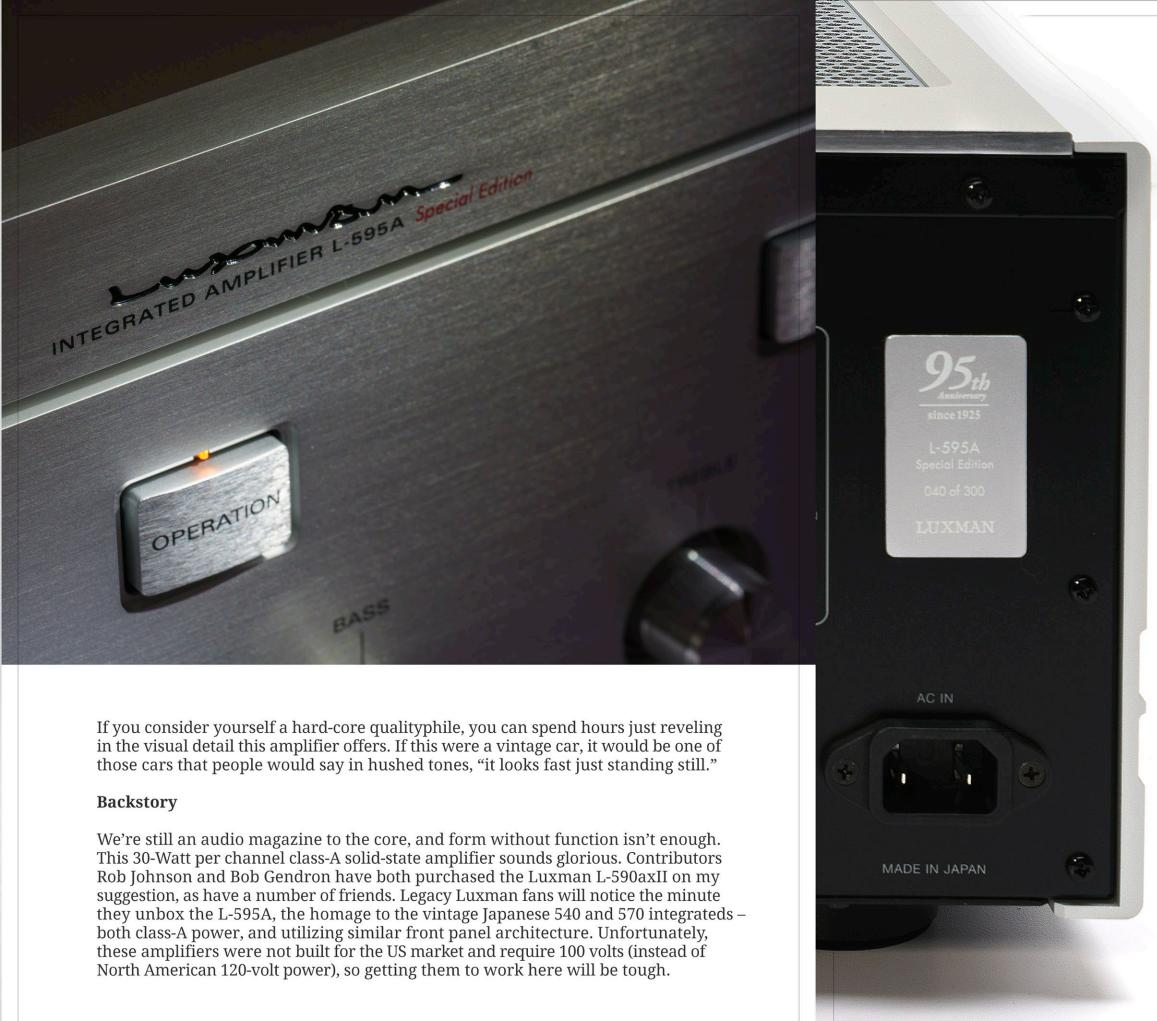
For those thinking this is merely an L-590aXII with a few tweeks and no meters, the difference is much greater. Luxman says using the pushbuttons instead of a rotary dial result in a quieter circuit – which you will also notice the minute you turn the L-595ASE on. It is even quieter than what you are used to with Luxman amplifiers. And the individual switches are unique to this model.
