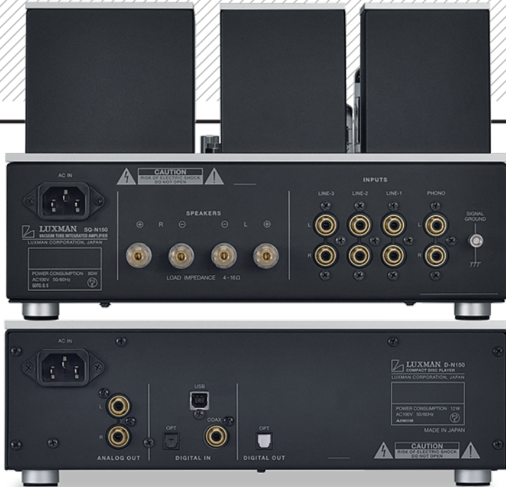
ABOVE: Three line ins and MM phono (on RCAs) join single sets of (switched) 4mm speaker cable terminals on the amplifier [top]. The CD player [bottom] has analogue (RCA) and optical digital outputs alongside coax, optical and USB-B digital inputs
