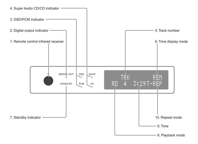
1. Remote control infrared receiver / R Receives the infrared signals from the remote control.
