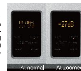
At normal At zoomed Zoom mode display at normal or zoomed mode
